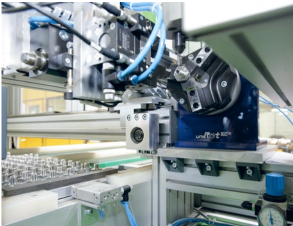
Labelling of pressure-bearing components
